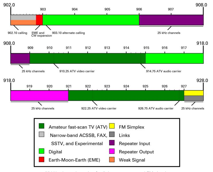
25 kHz channel spacing for links, repeaters, and FM simplex Two digital channels 3 MHz wide each, duplex pair Two ATV simplex channels 6 MHz wide each
